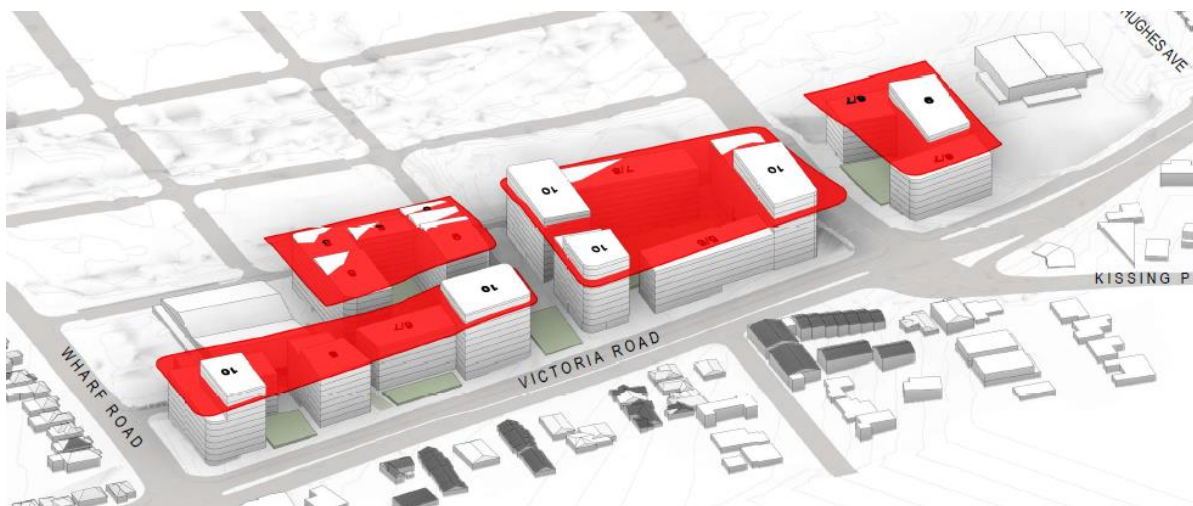
Figure 9. Building Envelope Height Breaches as proposed (28m building height plane in red).
